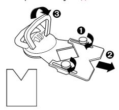
It is impossible to drill without a drill guide. (see page 9). You can improvise a drill guide using a piece of wood or plastic. Make a V-shaped insertion like illustrated and tape or clamp the guide onto the tile in the desired position.
